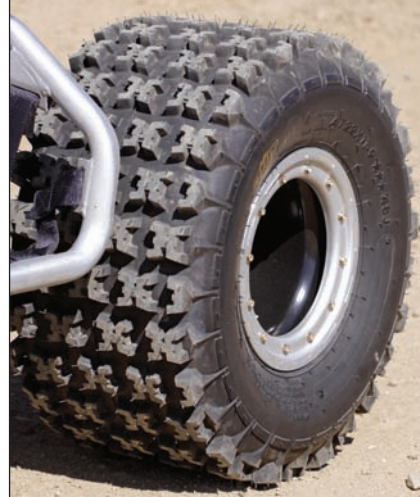
The 12-ply DWT tires are literally bullet-proof. The team tested the tire with no valve-stem cores (no air in the tires).
