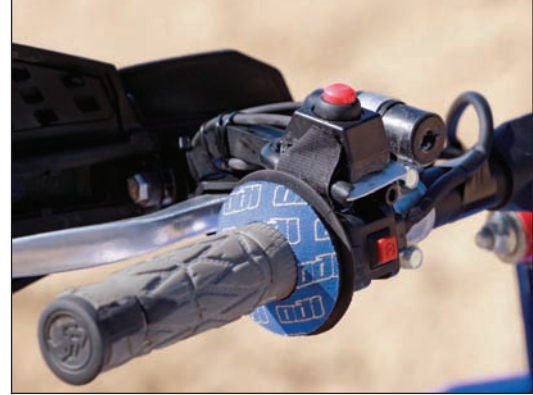
Spider grips with ODI donuts grace the Fasst Co. Flex bar ends, as well as a plug for the communication system and a talk button for the radio.
