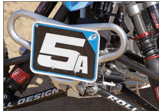
The GPR stabilizer (behind the front bumper) helps keep steering kick down. Here you can see the start of the plastic GYTR frame skid plate and the GYTR bumper with number plate.
